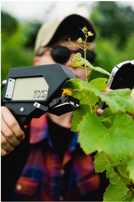
Capturing spectral measurements of a grape leaf using a Leaf Clip and Reflectance Probe. Photo credit: Cornell CALS marketing.
